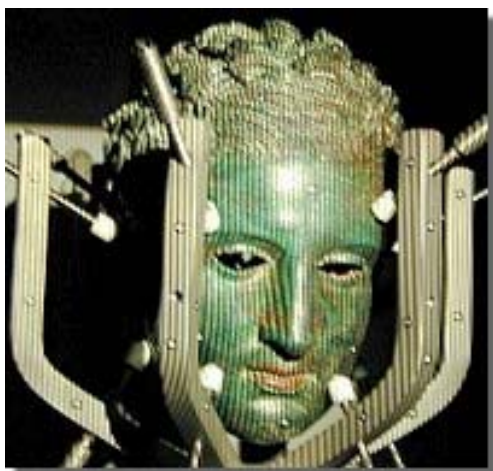
Fig. 4 Digitizing of the Apoxyomenos head with ATOS II - the projected fringe pattern and the reference markers are visible
