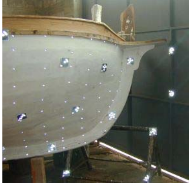
Fig. 3 Preparation of the bow for photogrammetric recording.
