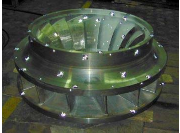
Fig. 8 Preparing the rotor for 3D scanning
