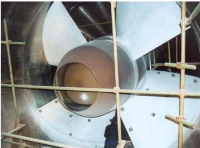
Fig. 13 Preparation of the turbine wheel (5.4 m diameter) for 3D scanning
