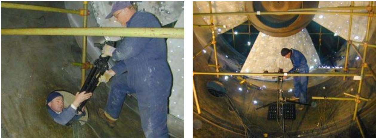
Fig. 1 The measuring systems ATOS and TRITOP are passed through a small opening into the turbine of a hydroelectric power plant. This allows for measuring and assessing the installed turbine rotor.
