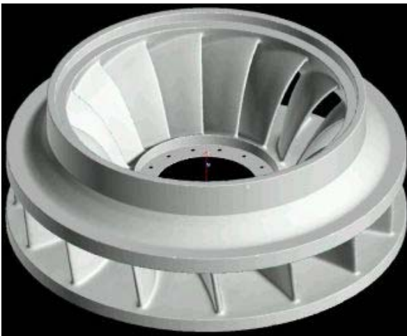
Fig. 9 3D scan of the rotor of a Francis turbine
